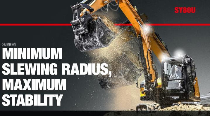
The SANY SY80U reduced tail swing excavator is ideal for large-scale loading projects or work in confined spaces. Thanks to the compact reduced tail design with minimal rear swing radius, the operator can work safely in tight spaces or directly in the vicinity of obstacles.
