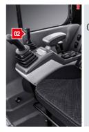
02 Once the operation is selected, use lever to adjust to the desired track width
