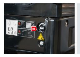
01 Battery Isolator is located on the front left corner of the cab. The horizontal position in **ON**. The vertical position in **OFF**.
