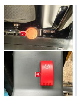
01 The Emergency Stop Switch is located by the cab door, or in the left hand arm console and displays as a Rocker Switch. Pulled out is machine **ON**.
