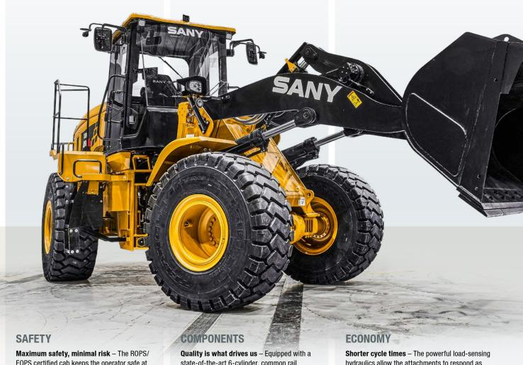
Maximum safety, minimal risk – The ROPS/FOPS certified cab keeps the operator safe at all times and the 360 camera system ensures an unrestricted view when working. To protect bystanders a travel alarm and rotating beacon is also fitted on the machines as standard.
