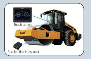
Real-time detection of compaction parameters (ICV compaction value, amplitude and vibration frequency).
